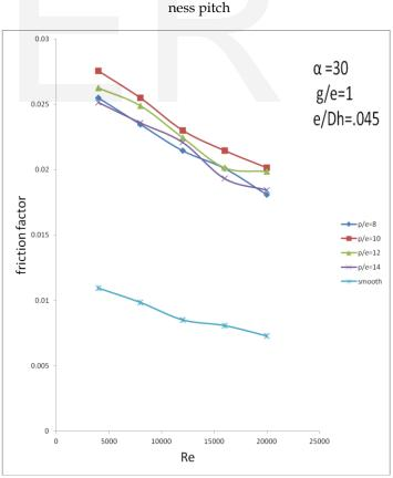
Fig .4.5 Friction Factor and Reynolds no. with different rough-
