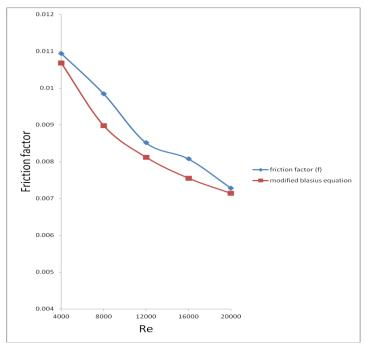
Fig .4.3 Friction factor .and Reynolds no. cfd & modified blasius equation
